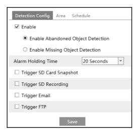
1. Enable abandoned/missing object detection and then select the detection type.
