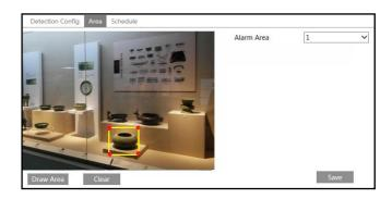
Set the alarm area number and then enter the desired alarm area name. Only one alarm area can be added. Click the "Draw Area" button and then click around the area where you want to set as the alarm area in the image (the alarm area should be a closed area). Click the "Stop Draw" button to stop drawing. Click the "Clear" button to delete the alarm area. Click the "Save" button to save the settings.
