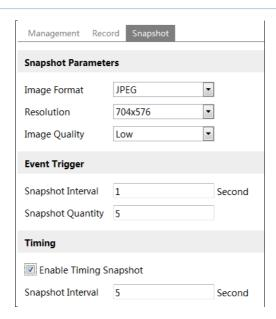
Set the format, resolution and quality of the image saved on the SD card and the snapshot interval and quantity and the timing snapshot here.
